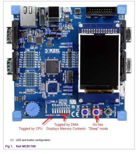
A block of unused memory is cleared and configured with known data. In this case we will configure the SRAM to contain incrementing values. These values are then displayed on the LEDs which are controlled by the DMA.
